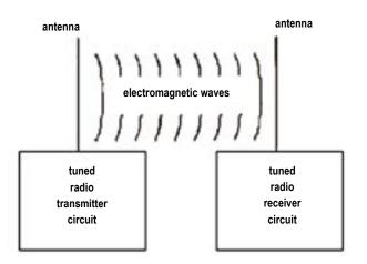
Figure 2. Radio Transmitter and receiver (resonance)
